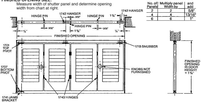
1. Cut track precisely to fit finished opening. Locate pivot lock so that center of pivot is 15/8" from end of track, and tighten in track. Unlock pivot by moving lock tab towards end of track. Insert wheeled part of each hanger as needed and insert snubber at end with rubber bumper facing pivot. Mount track in center of header.
