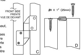
FASTEN PIVOT PLATES to top and bottom of doors as shown.
