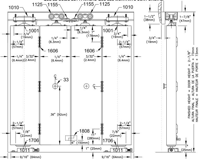
**CUT TRACK TO FIT OPENING WIDTH** and fasten to header jamb with 1-1/4" (32mm) pan head screws. NOTE: INSERT PARTS IN TRACK BEFORE MOUNTING.
