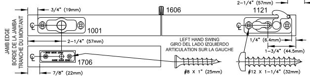
**FASTEN 1011 FLOOR BRACKET** to floor 9/16" (14mm) from jamb face and 7/8" (22mm) from jamb edge. Remove floor bracket and proceed to Step 5.
