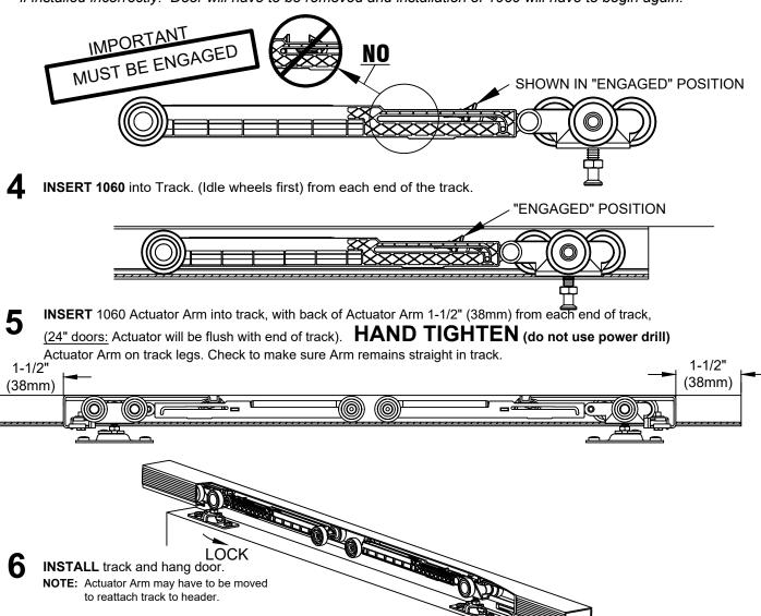
**SLOWLY** slide door toward Jambs, checking to make sure door touches Jamb, if not. Slide door away from Jamb and readjust Actuator Arm. Slowly close door again, checking to make sure soft close is working properly. Once confirmed, begin using door normally.
