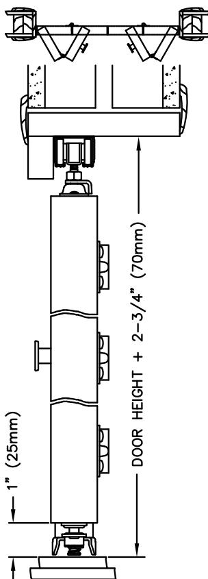
A deluxe commercial grade, folding door hardware set designed for use with heavy  $\frac{3}{4}$ " to 1 $\frac{3}{4}$ " doors weighing up to 50 lbs. per door panel.
