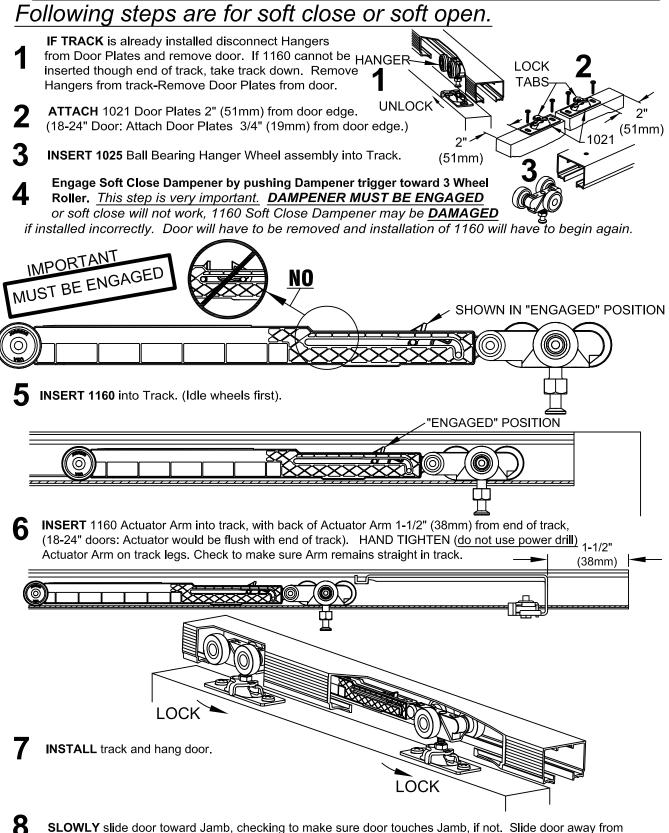
**SLOWLY** slide door toward Jamb, checking to make sure door touches Jamb, if not. Slide door away from Jamb and readjust Actuator Arm. Slowly close door again, checking to make sure soft close is working properly. Once confirmed, begin using door normally.
