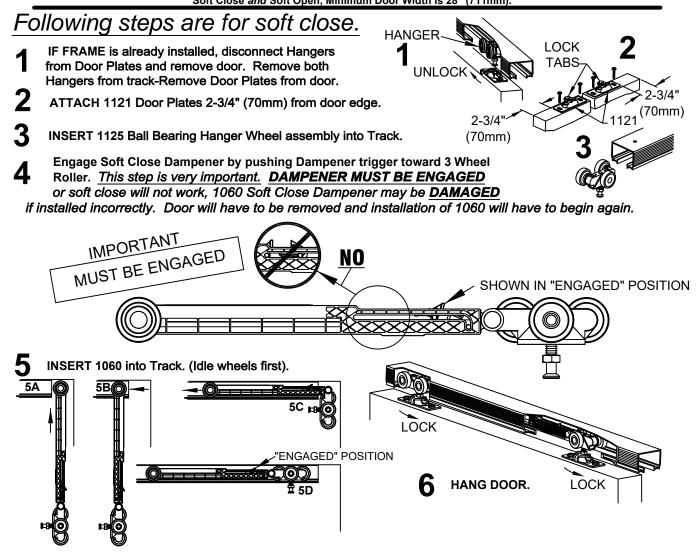
SLIDE door away from end of track (check to make sure all track screws are flat against track) and install 1060 Actuator Arm into track, with back of Actuator Arm 2-1/4" (57mm) from Jamb.
